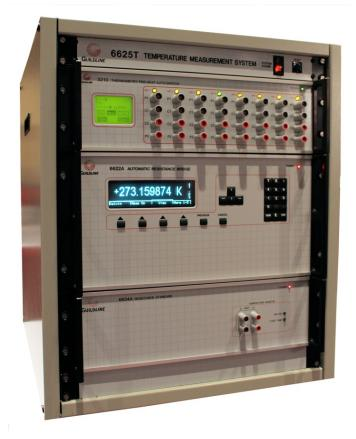
The 3210 Thermometry Adaptor provides automation support for the calibration of multiple PRTs, SPRT's or other thermometer devices.
